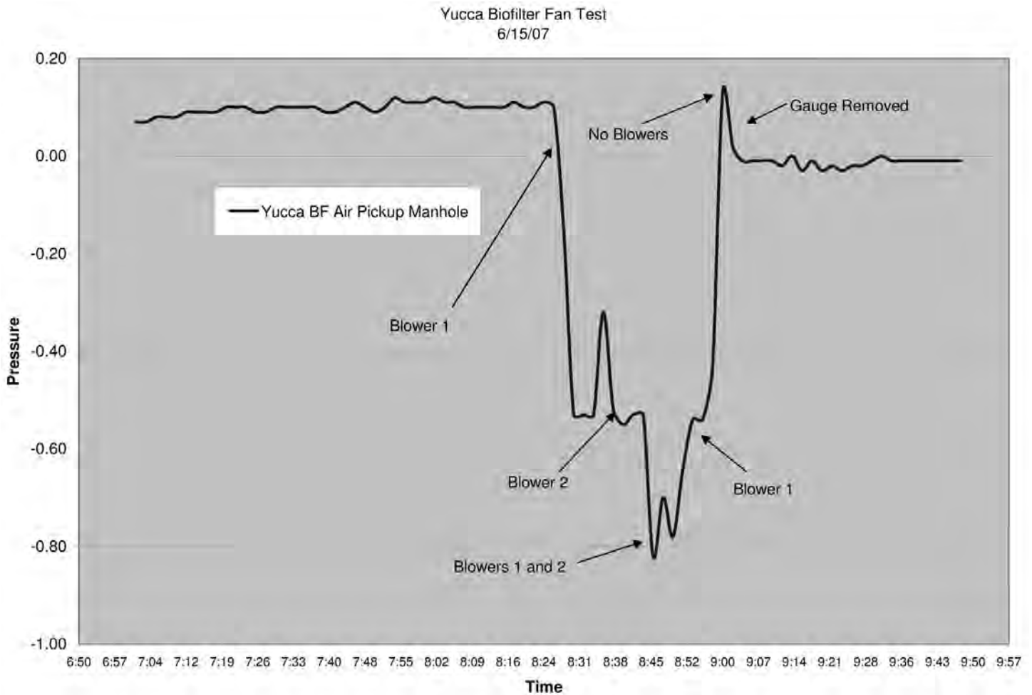
Figure 2. Air Pressure Data with Forced Air Ventilation
