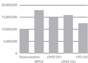
Figure 2. Net present worth for pasteurization and UV systems
