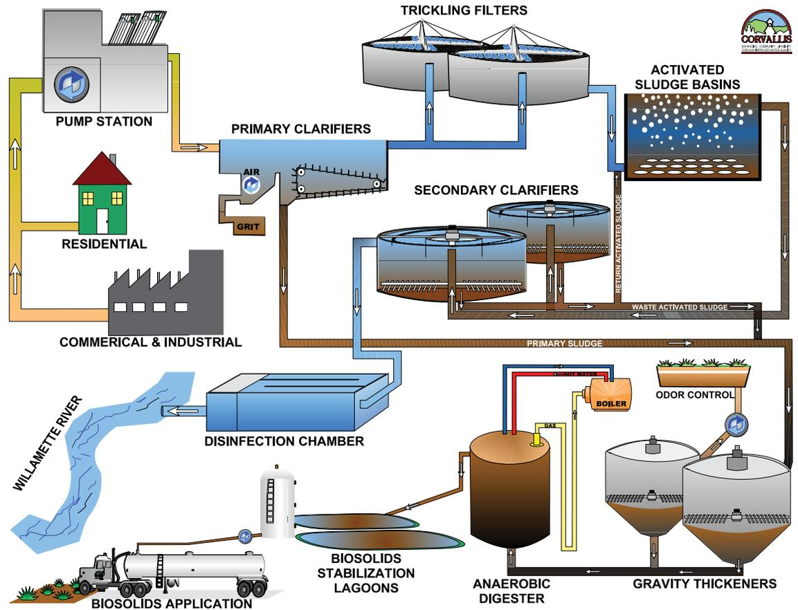
Corvallis WWTP schematic (does not show nutrient recovery)
