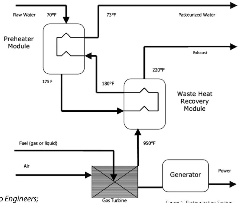
Figure 1. Pasteurization System
