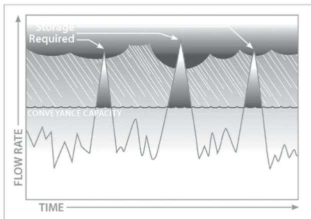
maintenance. However, active controls including float gates, motor operated gates, inflatable dams, pinch valves and pumps will provide better flexibility in operating the storage, and in most cases, can reduce the size of the tank while providing the same protection as a passively operated facility.
